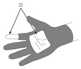
1 3 in. (76 mm) square cut out and finger of glove cut off
